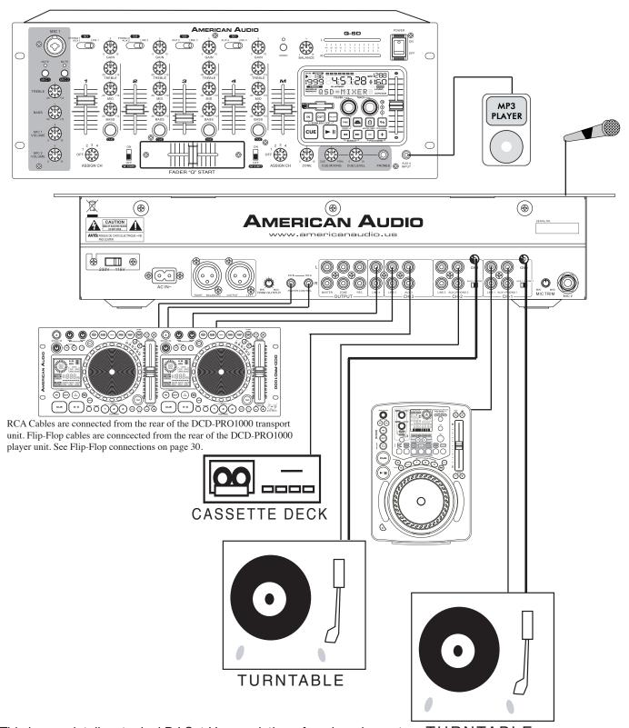
This image details a typical DJ Set Up consisting of a microphone, turn-TURNTABLE tables, CD players, and a tape deck.
